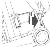
6. Lift agitator assembly out and remove worn belt.
